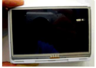
Connect communications cable to rear of screen, and clip screen into cover mounted in wall.
