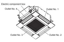
The outlet No. is indicated by the number of grooves on both ends of each air outlet. Set the air direction while checking the information shown on the remote controller display.
