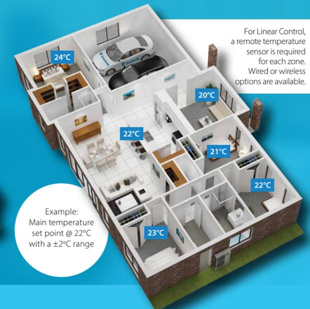
For Linear Control, a remote temperature sensor is required for each zone. Wired or wireless options are available.
