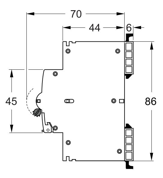
NHP MOD6 Residual Current Device - Short body w/ Overcurrent 6kA 20A 1PN C Curve 30mA Type A Pigtail
